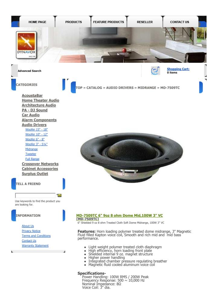
Magnet Weight: 9 oz. Sensitivity: 94dB W/M Fs: 450 Hz Re: 6.2Ω
